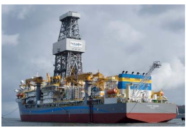
Dual derrick, offline handling & rig floor automation
